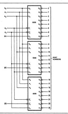
Figure 2, I/O Port Decoder
